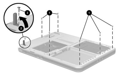
Removing the Display Panel Assembly Screws
